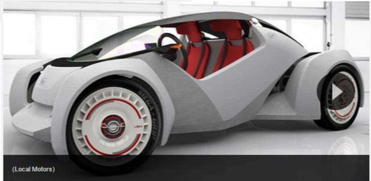
STARTI is an [electric car](#) developed by [Local Motors](#) and manufactured in collaboration with [Cincinnati Incorporated](#) and [Oak Ridge National Laboratory](#).<sup>[2]</sup> It is the world's first 3D-printed electric car.<sup>[3]</sup> The car was manufactured using a Large Scale 3D Printer developed by [ORNL](#) and Cincinnati Inc. The car took just 44 hours to print during the 2014 [International Manufacturing Technology Show](#) in [Chicago, Illinois](#).
